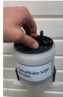
Step 6. Place new motor piston carefully into pump body and replace lid.
