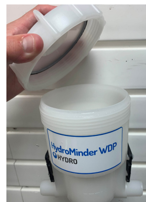
Step 9. Replace lid onto the pump body. Ensure o-ring is still in the lid before putting it back on.
