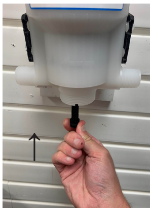
Step 7. Place shaft into the motor piston and rotate shaft 90° to lock into place. Gently pull down to ensure shaft is locked.
