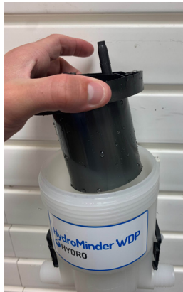
Step 5. Remove motor piston from pump body.
