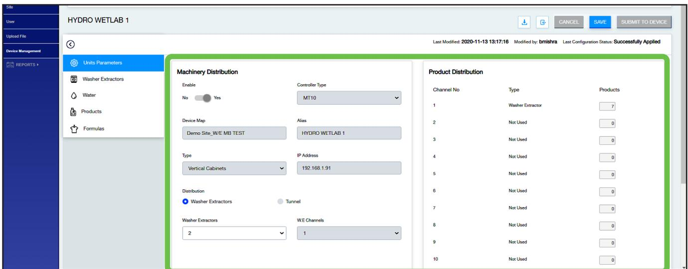
This section outlines the basic parameters of the dispensing system. Most of the fields in this section are not editable and are grayed out, indicating they are read-only. Each field is described in more detail below:
