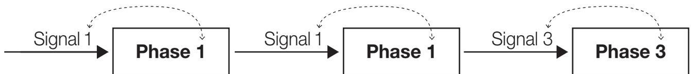
**Mixed Sequential Mode:** Works the same as Sequential mode, but it requires exclusively signal 3 to advance to the third phase. See the example below:
