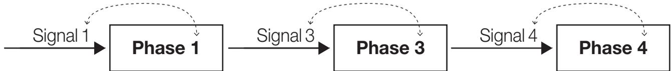
**Sequential Mode:** Every time signal 1 or 2 is received, the unit advances one step in the formula and doses the products associated to it. Just for the first phase, we can also use signal 5. (E.g. we can connect a filling valve to signal 5.) The reception of signal 5 after having executed the first phase has no effect. See the example below:
